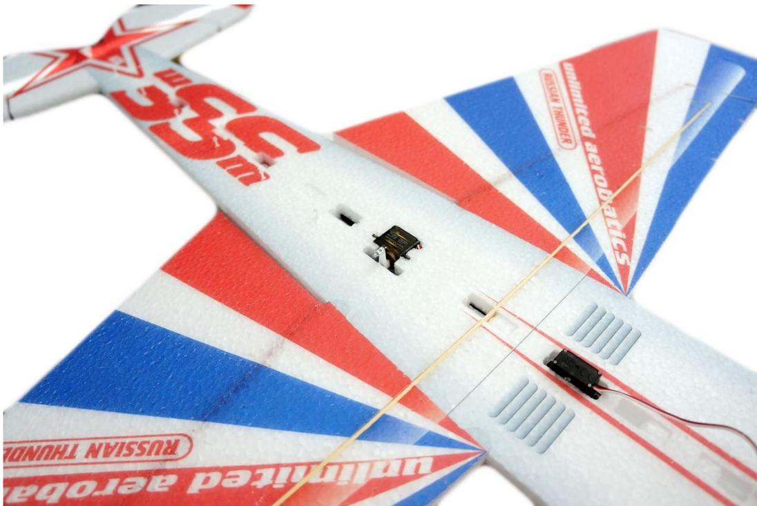
Secure the lever with a screw. Press on the soft EPP with a screwdriver and bend it to the side so you can screw the screw.
