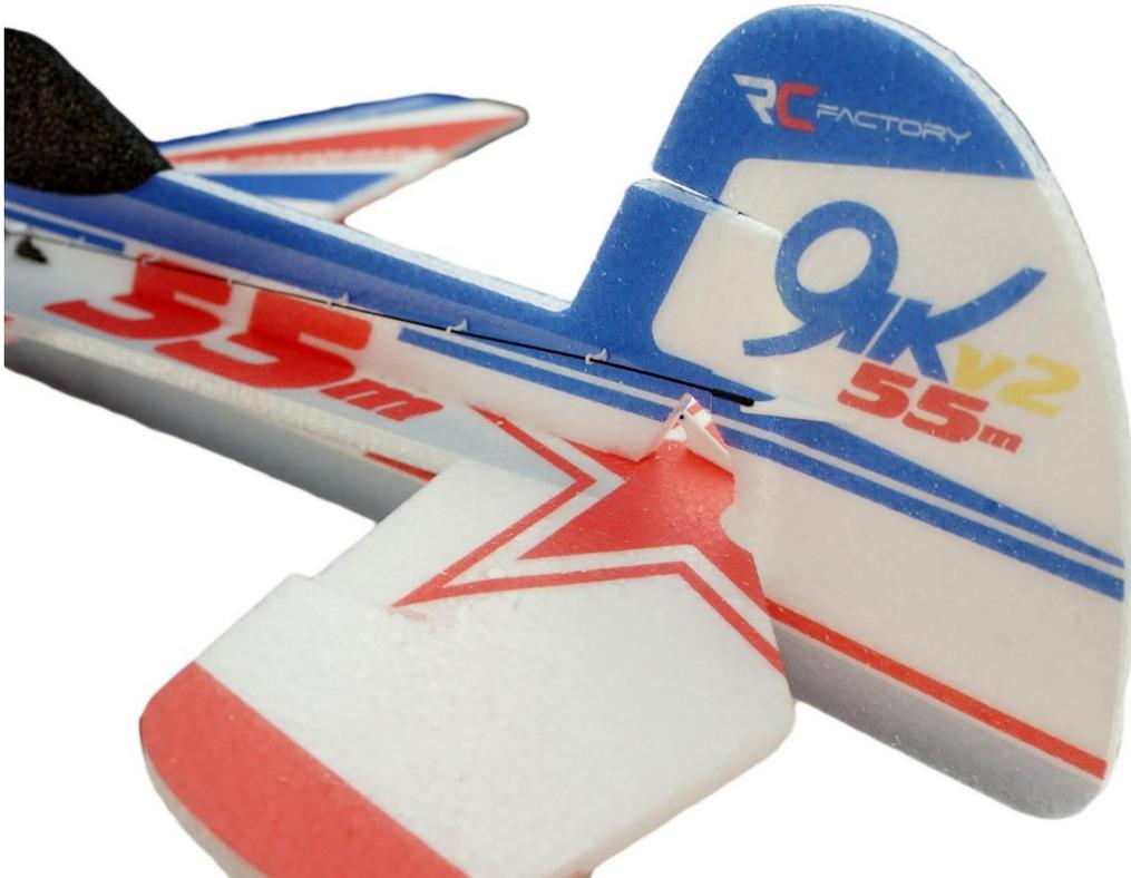
Align the rudder to the straight position. Make sure that the servo lever is perpendicular to the top of the airplane and lock the rod with a screw. Shorten the excess length of the rod.
