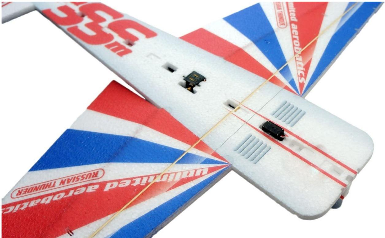
Put together the lever for the servo to control the ailerons. The package includes more 3D printed parts for use with other types of servos. The wider part of the lever goes to the place marked by the groove. Take a lever from the D14M servo and insert it into the prepared 3D print. Apply some glue and cover the lever with the smaller 3D printed part.
