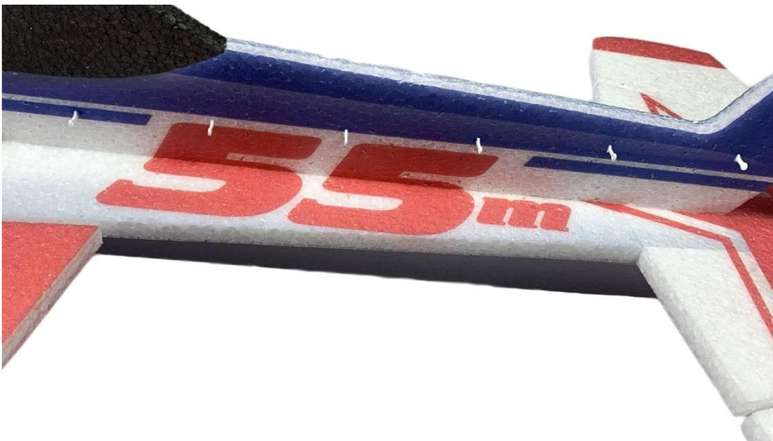
Starting from the rudder, stretch the entire rod through the guides and blimp on the servo lever. Click the end fork into the lever on the rudder.
