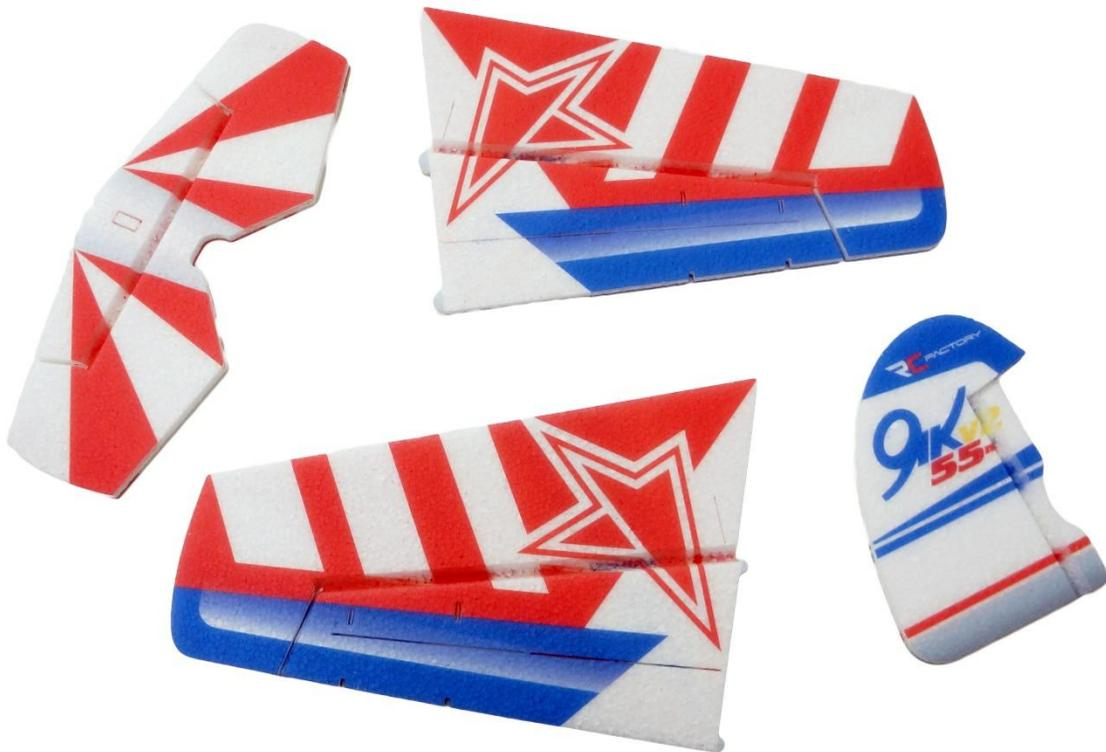
Fold the parts and load them evenly. You can use books, for example. Leave the parts for about 1-2 hours. In the meantime, prepare a space to build the plane. You will need a free table. Since the plane is primarily glued, it is good to cover the table with a piece of plastic, which will protect the table and prevent the airplane from sticking to the table.
