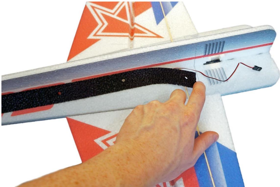
Turn the plane over and insert the Volta DM14 servo, which will control the ailerons. Stretch the cable to the underside of the airplane. Then secure the servo from the sides with glue and spray it with an activator.
