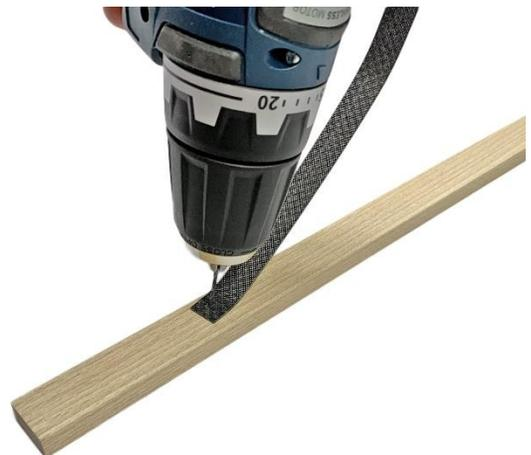
Roughen the laminate parts from one side with sandpaper. On a roughened surface, glue will hold better.
