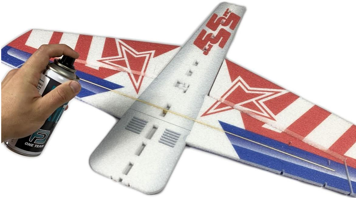
Next, install the elevator. Spray the elevator with an activator, apply glue to the central part and press tightly. There are protrusions on the elevator and the central part, thanks to which it should not be possible to glue the elevator in reverse.
