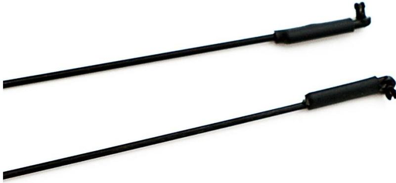
Stretch the elevator rod through the guides to the servo lever through the blimp. Then click the fork into the elevator lever from the outer side.
