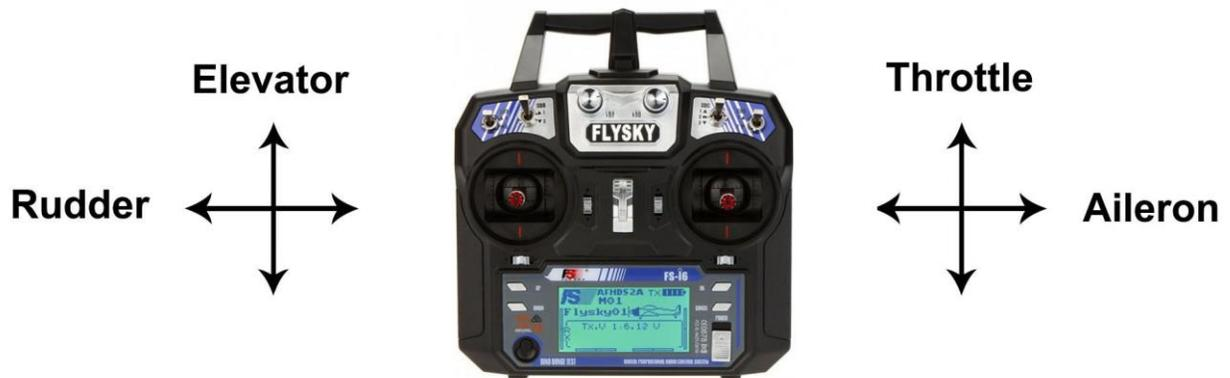
When the right gimbal is deflected to the right (leave the throttle at the bottom), the right aileron must be raised and the left one lowered.
