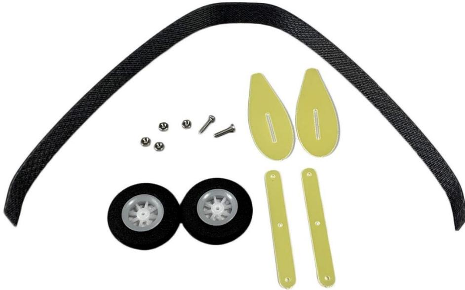
Take the carbon landing gear, laminate wheel holder and wheels. Enlarge the hole with a two-millimeter drill in the laminate holder and in the wheel. Drill a hole on both edges of the carbon landing gear. The hole should be about 4mm from the edge.
