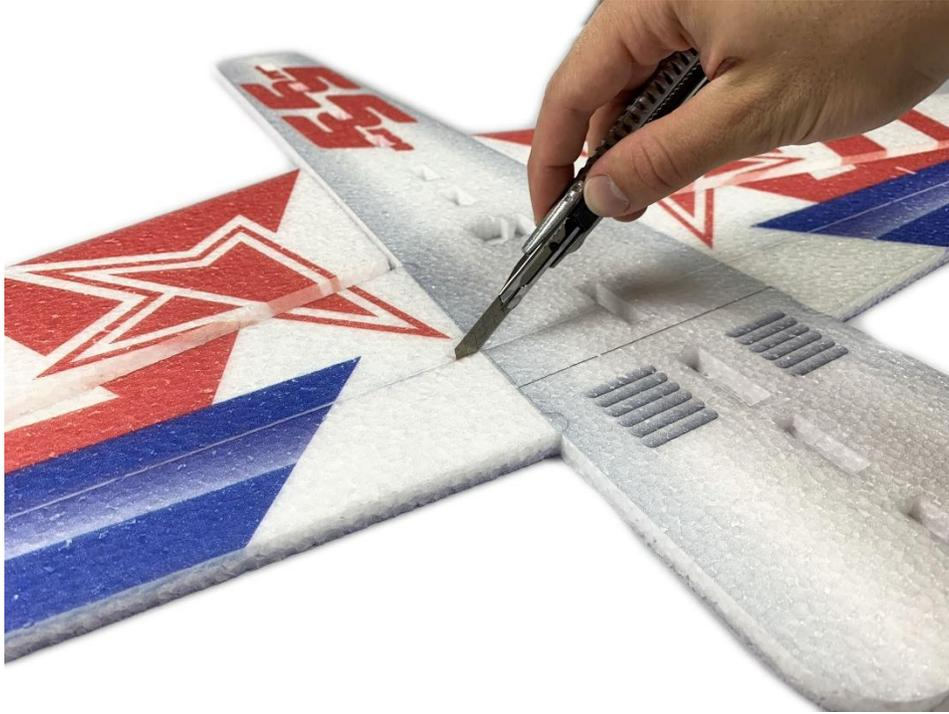
Apply glue to the reinforcement from both sides, insert it into the groove, spray it with an activator and press the EPP around it firmly.
