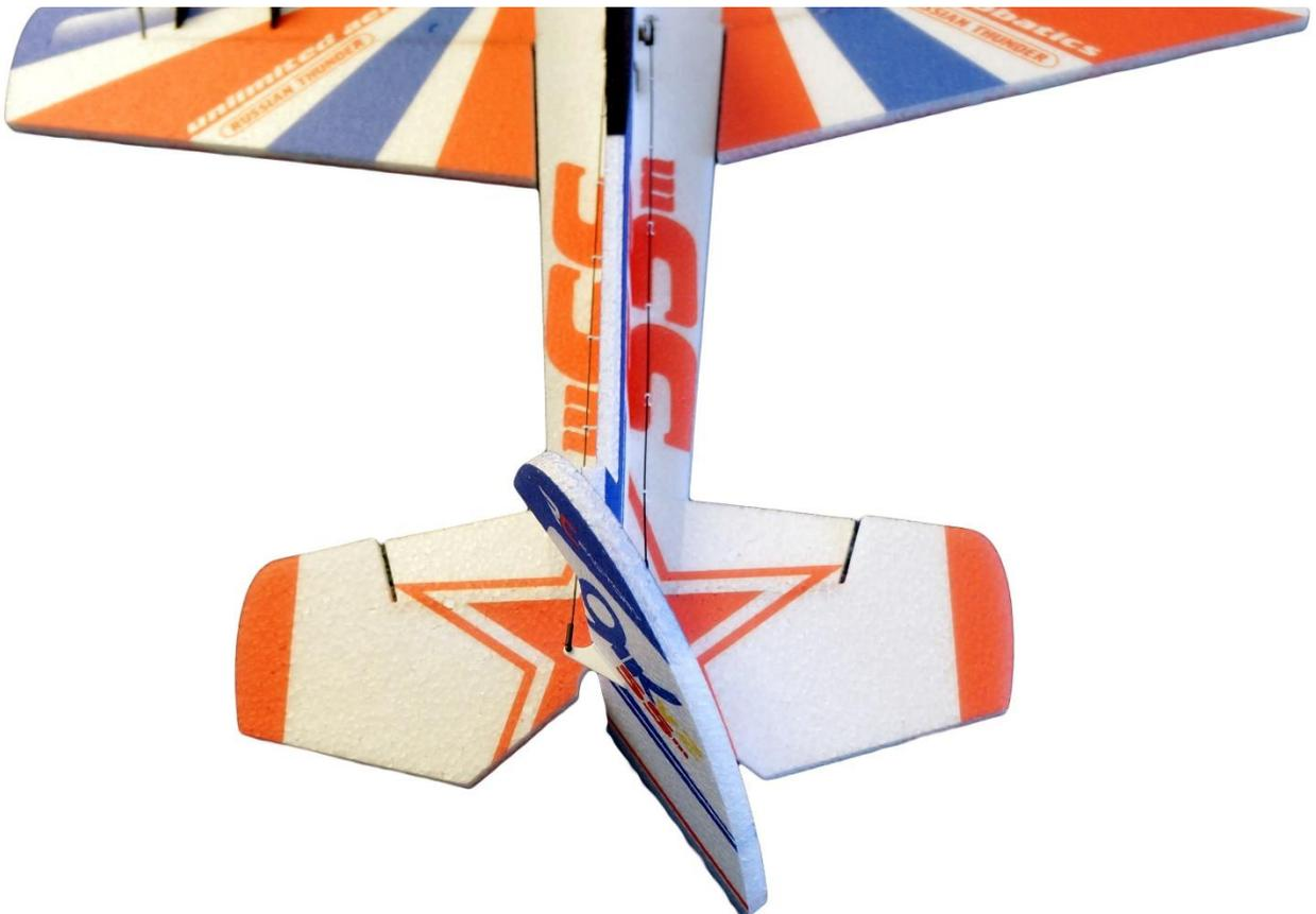
When the left gimbal is deflected downwards, the elevator rises upwards.
