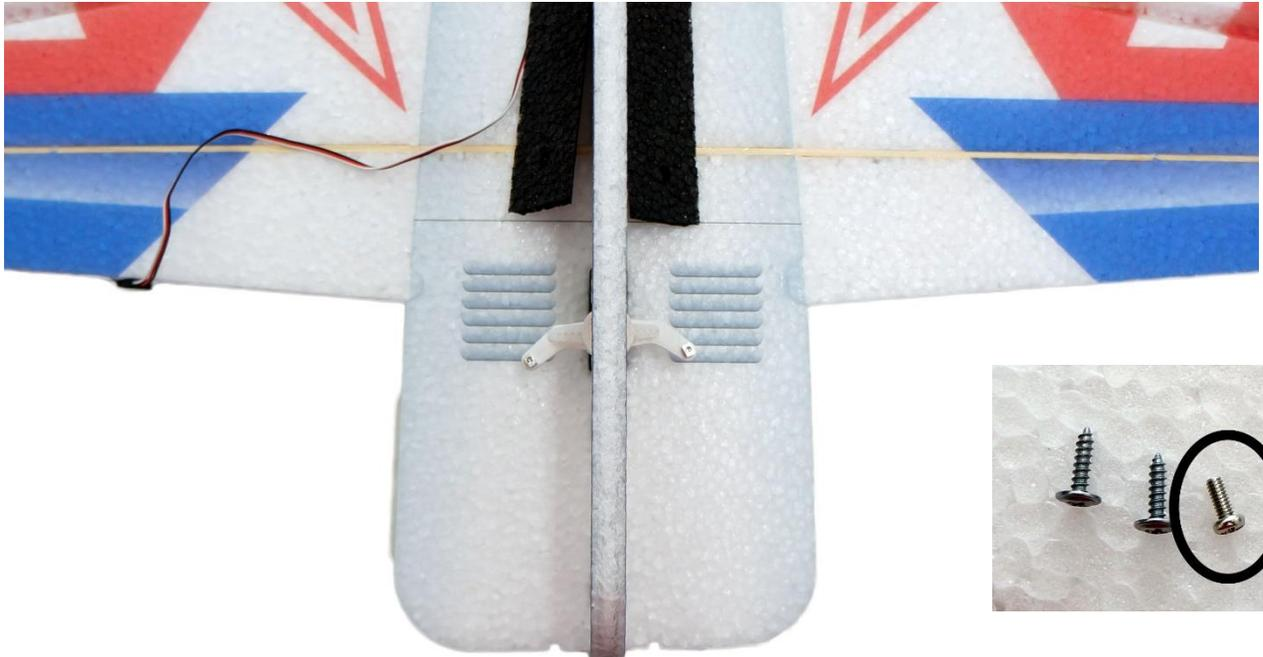
Finally, lock the lever with a screw. Select a smaller metric screw from the package. Press the EPP with a screwdriver and bend it to the side so that you can screw the screw in.
