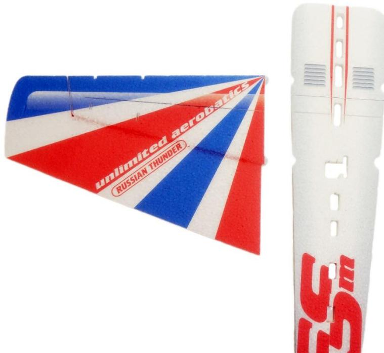
Let's start with gluing the wing. The wings have differently sized semicircular protrusions. Therefore, it should not happen that you glue the wings in reverse. Apply the activator to the middle part of the plane and glue on the wing then press them firmly together. Be careful not to glue the ailerons. We apply the same procedure to the second wing.
