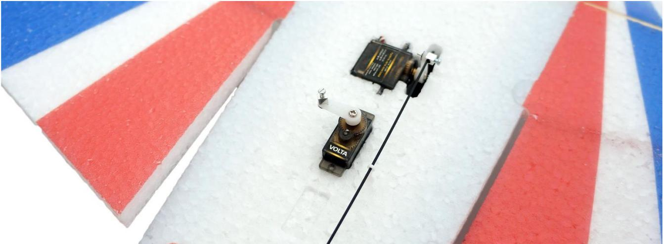
Prepare the upper part of the airplane. Apply glue to the black cabin, spray the upper part with an activator and press them together.
