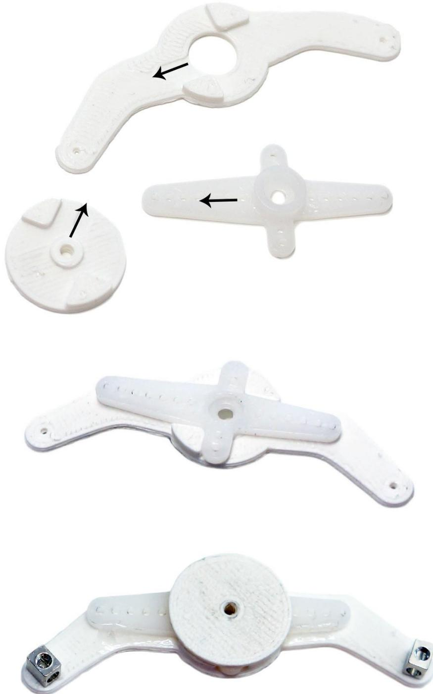
Now put blimps (that metal thing with a pin) into the 3D printing according to the pictures. Secure the blimp sufficiently with snap ring so that it does wiggle, but it can be rotated freely. The snap ring goes to the pin stiffly, so you need to use a little force.
