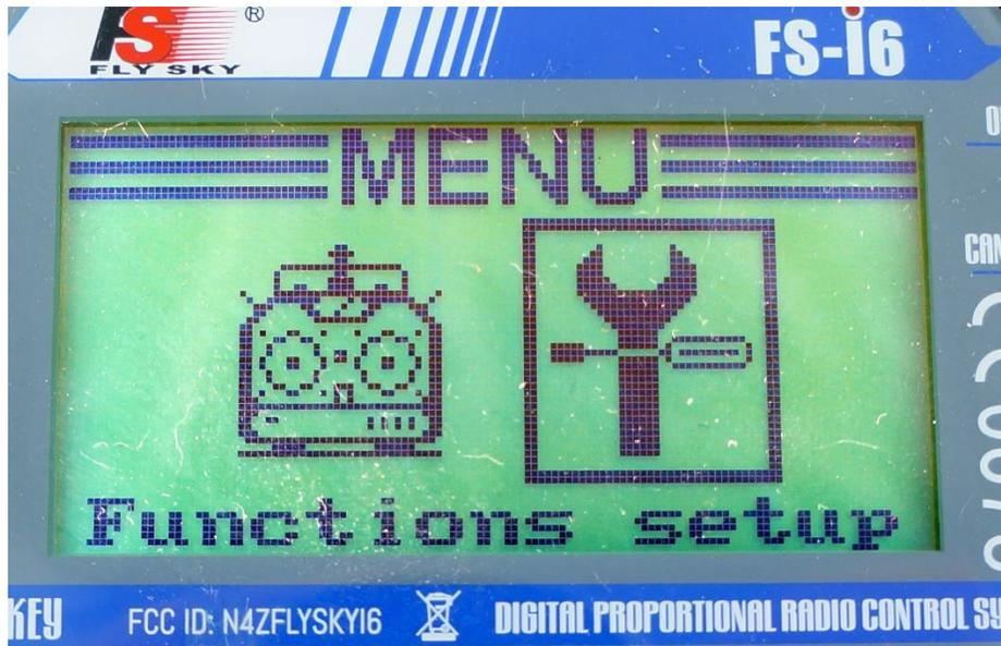
Press the **Down** button to go to the **Dual rate/exp.** option and confirm with the **OK** button.
