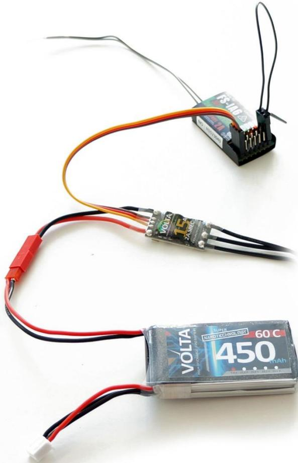
Now connect also the servos to the receiver (one is missing in the picture). We will use the first 4 channels CH1, CH2, CH3 and CH4. Then turn on the radio, put the throttle in the center position and plug the battery into the ESC. After connecting the radio with the receiver, the servos are centered.
