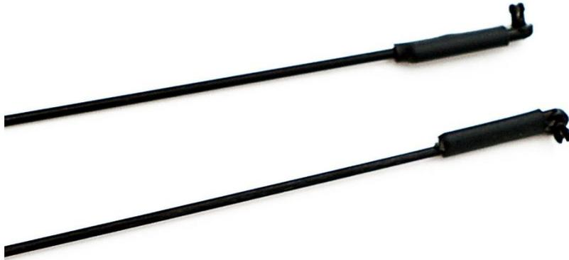
Stretch the elevator rod through the guides to the servo lever through the blimp. Then click the fork into the elevator lever from the outer side.
