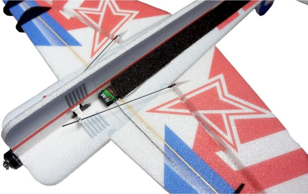
Mark the center of gravity of the airplane. COG should be 18 cm from the tip of the airplane. The center of gravity can be marked from the bottom with a marker.
