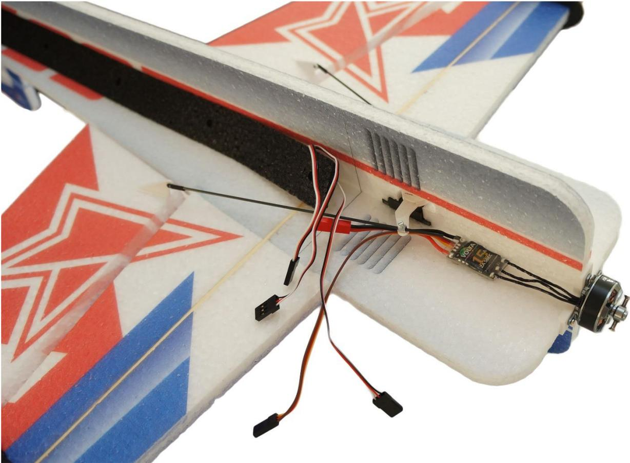
Finally, install the RC receiver. Place the RC receiver on the center of the airplane between the wooden reinforcement and the printed line. Mark the height of the receiver with a marker and cut a hole for the receiver in the EPP with a knife.
