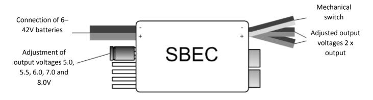
Wiring diagram of the regulator:
